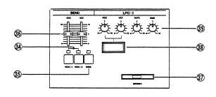
RISE TIME: This determines the time required for the LFO-2's modulation to reach the depth set by the BEND knob (36) in the Performance Control Section.
